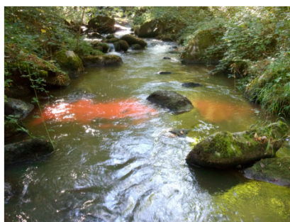
Figure 4. Photograph of the fluorescent orange sand tracers injected in the Selves River (Station 3) before the first release on September.
